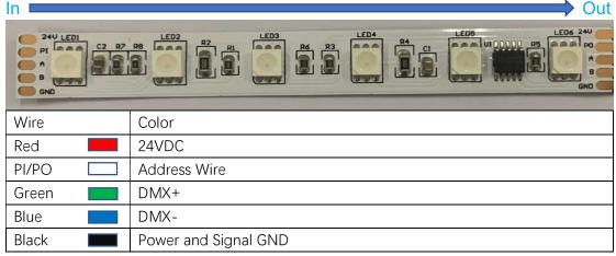
Note: Do not connect the Address wire for the first fixture.
