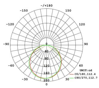
The Below curves indicate the illuminated area and the average illumination when the luminaire is at different distance
