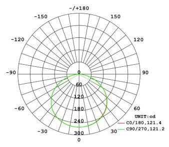
The Below curves indicate the illuminated area and the average illumination when the luminaire is at different distance((DS126003 DMX RGB Strip)
