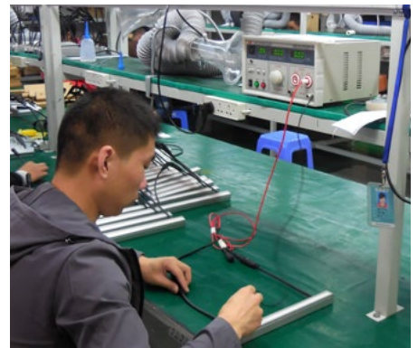
High Voltage Withstand Test
